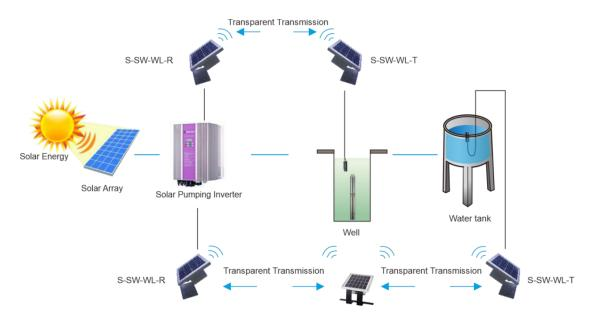
S-SW-WL Wireless Switch Signal Module is based on a point-to-point wireless communication module to realize long-distance transmission of switching signals. The longest effective communication distance can reach 2 km.
